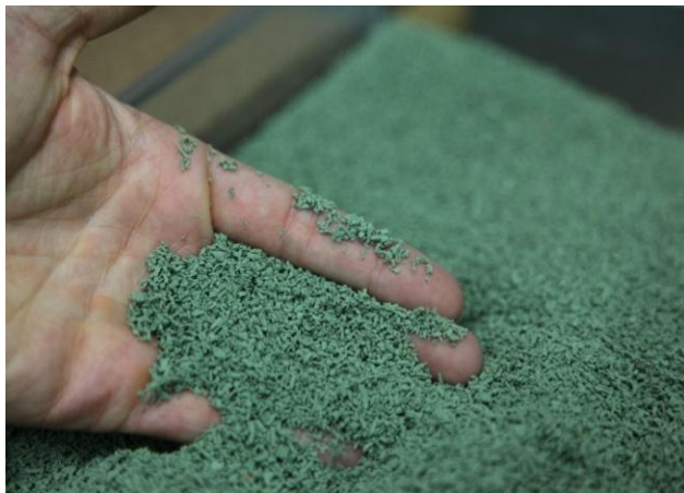
Photo 26: EPDM Infill (Source: Smart Connection Consultancy)
