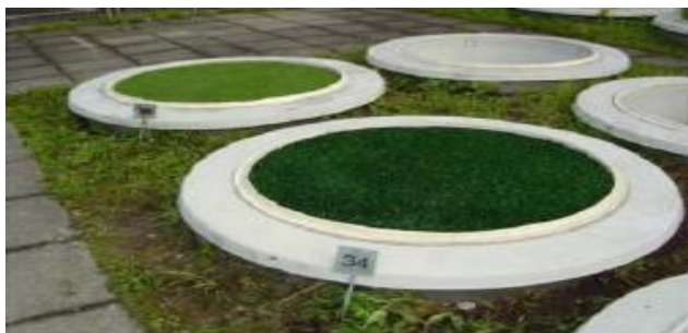
Photo 35: Swiss Study Collecting Rainwater Through Various Synthetic Sports Surface Systems
