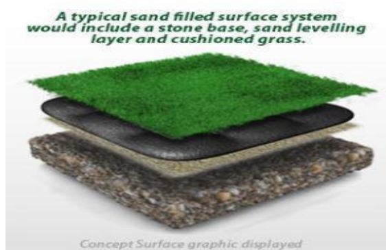
Figure 7: Sand Filled Carpet (source: ABS Sport Surfaces)
