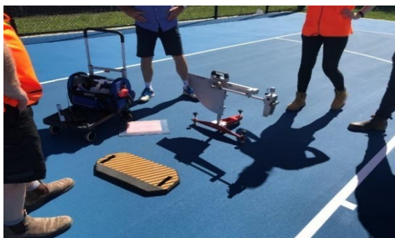
Photo 29: Testing Apparatus for Slip Resistance
