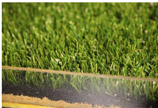
Photo 23: Example of a Mixed Profile of Sand And Rubber Infill
