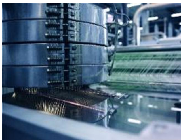
Photo 20: Extrusion Process Producing Mono-Filament Yarn
